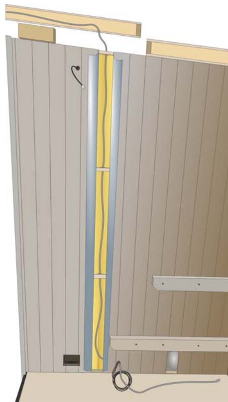
Figure 20. Routing Lighting Cable
