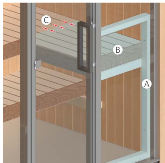
Figure 32. Installing Armrest and Return Bench
