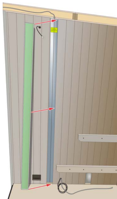
Figure 21. Taping Vapor Barrier and Installing Plank
