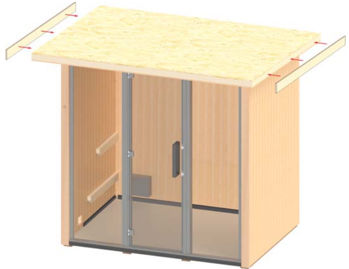
Figure 24. Installing Left and Right Side Wood Fascia
