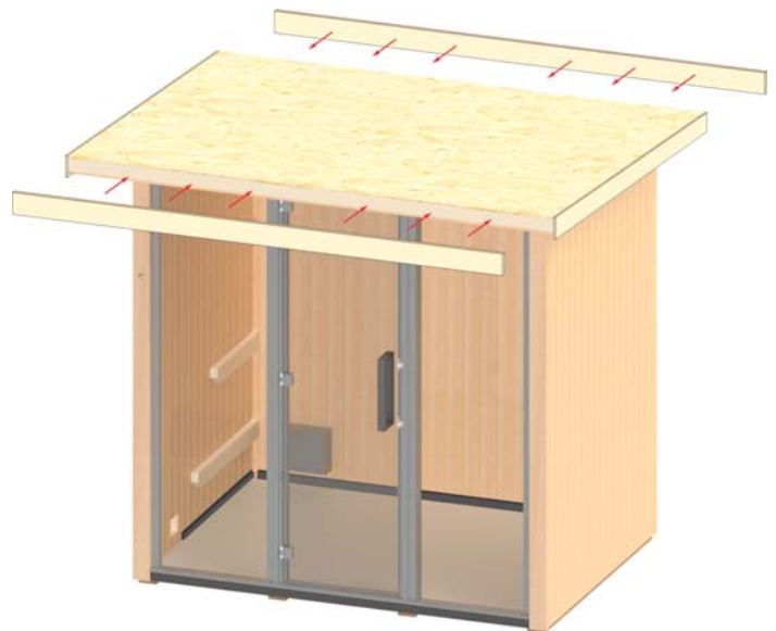
Figure 25. Installing Front and Back Wood Fascia
