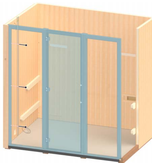
Figure 11. Installing Front Wall Frame Assembly
