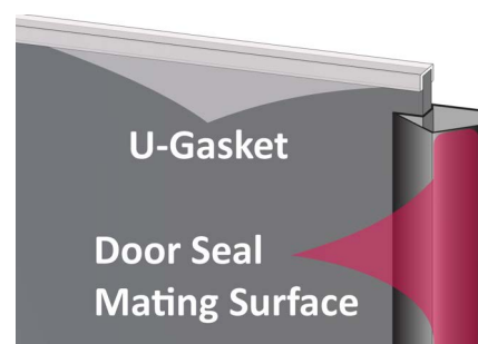
Figure 17. Single Glass Pane Orientation & U-Gasket
