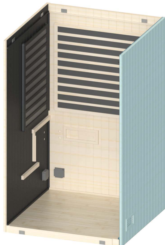
Figure 8. Installing Right Wall Section
