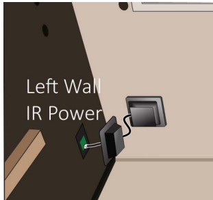
Figure 5. Left Wall IR Power Connection
