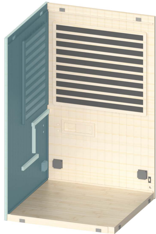
Figure 7. Installing Left Wall Section
