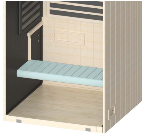
Figure 13. Installing Lower Bench
