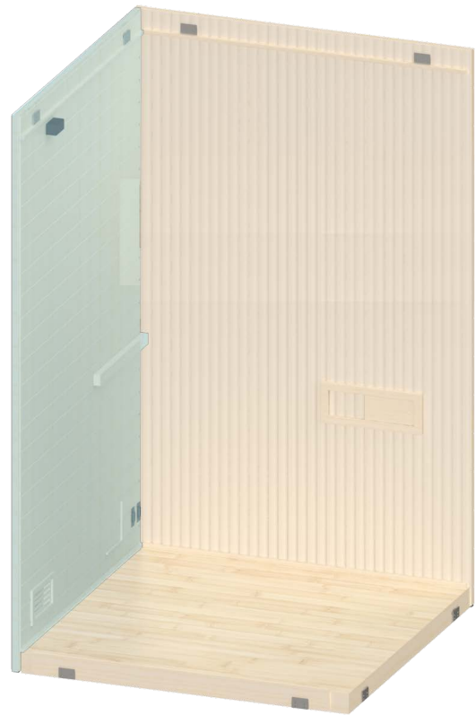
Figure 5. Installing Left Wall Section
