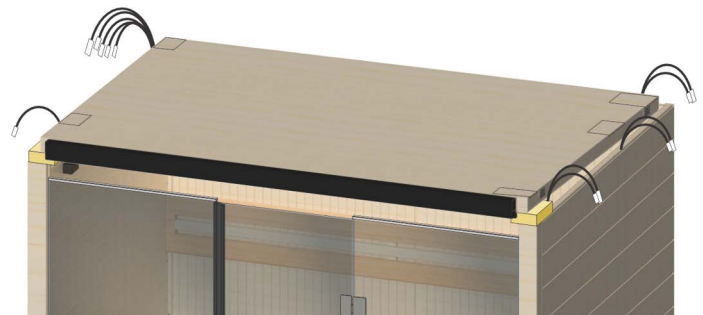
Figure 20. Preparing the Ceiling
