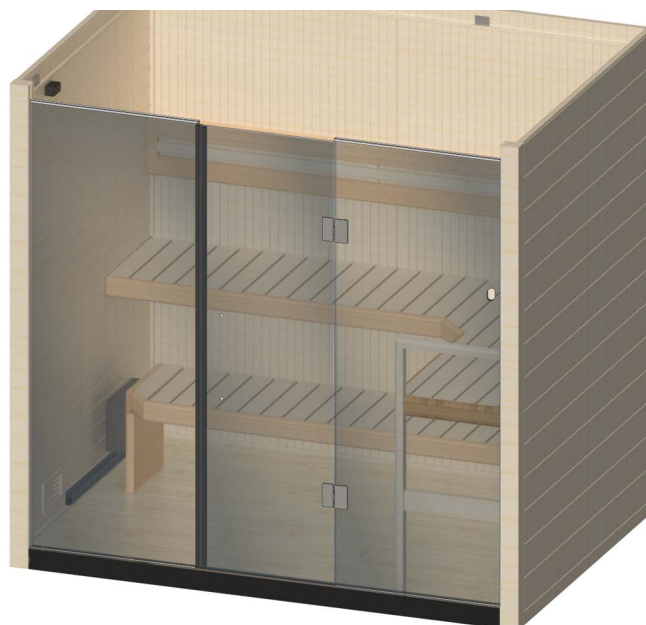
Figure 19. Installing the Door Assembly
