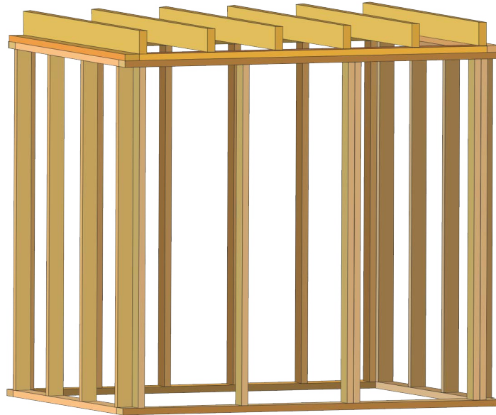
Figure 6. Example Framing for Horizontal Planks
