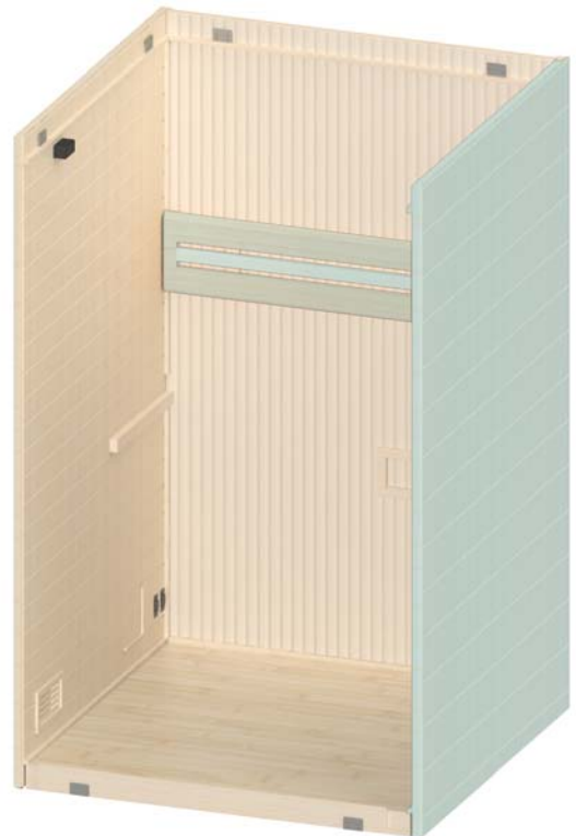
Figure 6. Installing Right Wall Section
