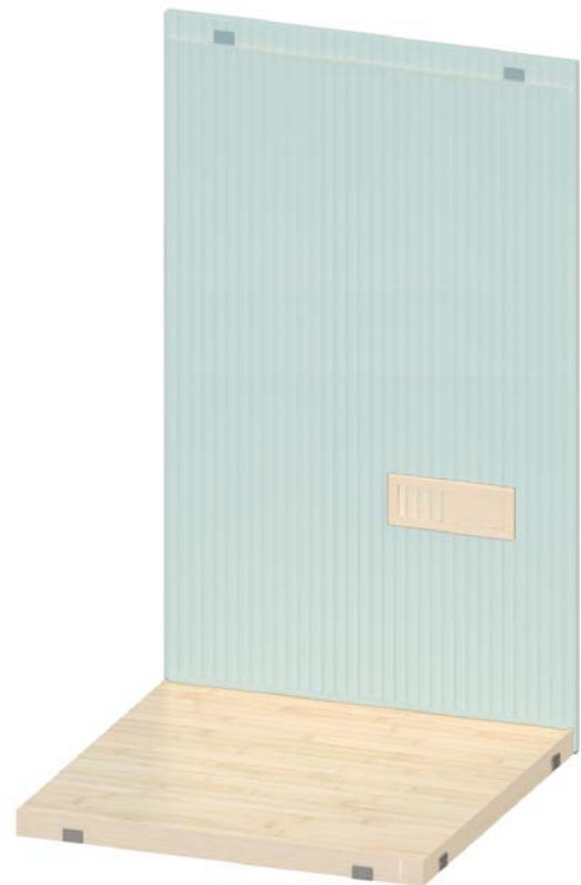
Figure 4. Installing Back Wall Section
