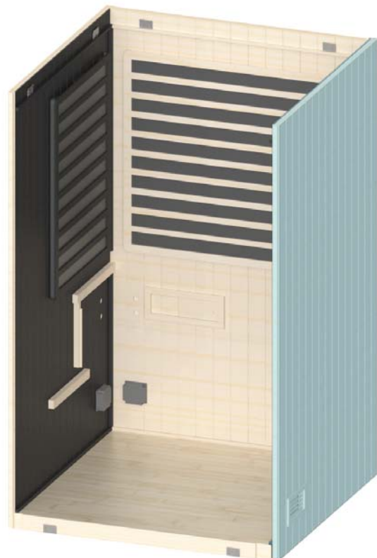
Figure 8. Installing Right Wall Section
