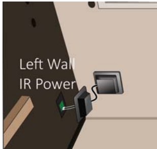
Figure 5. Left Wall IR Power Connection
