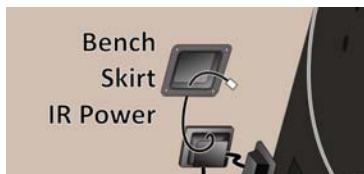
Figure 12. Bench Skirt IR Power Cable
