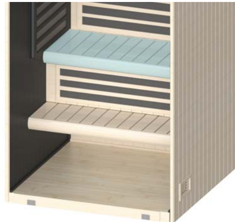
Figure 16. Installing Upper Bench Seat
