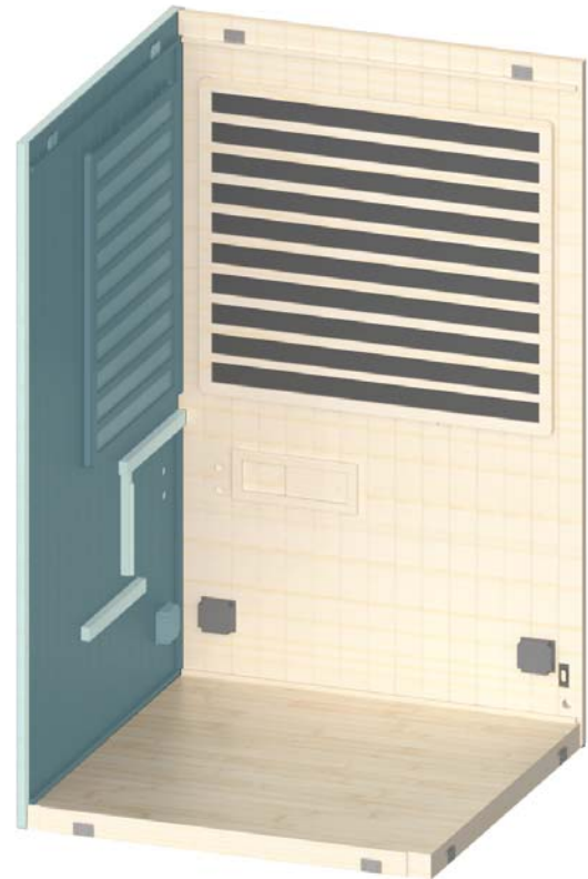
Figure 7. Installing Left Wall Section
