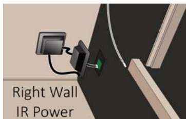
Figure 6. Right Wall IR Power Connection
