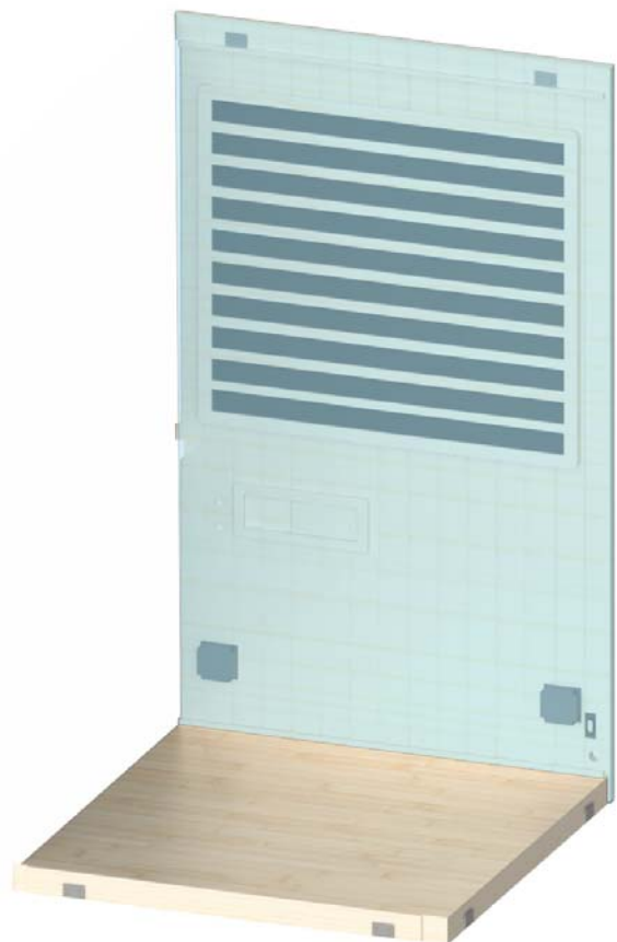
Figure 4. Installing Back Wall Section
